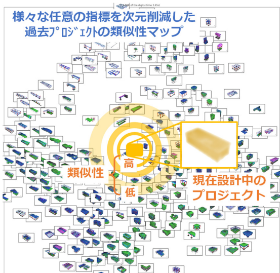
Figure 3. Application example of structural similarity map.
