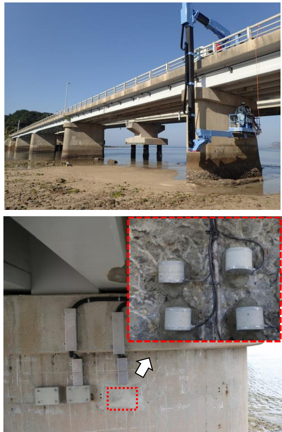
Figure 8. Verification experiment using optical Fiber Sensors
