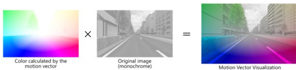
Figure 4. Composite of colors representing motion vectors and the original image (monochrome).
