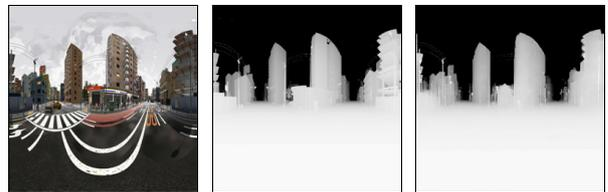
Figure 7. Example of a generated depth map of a test data by M2c, RMSE=4.37 (Center: original, right: generated).
